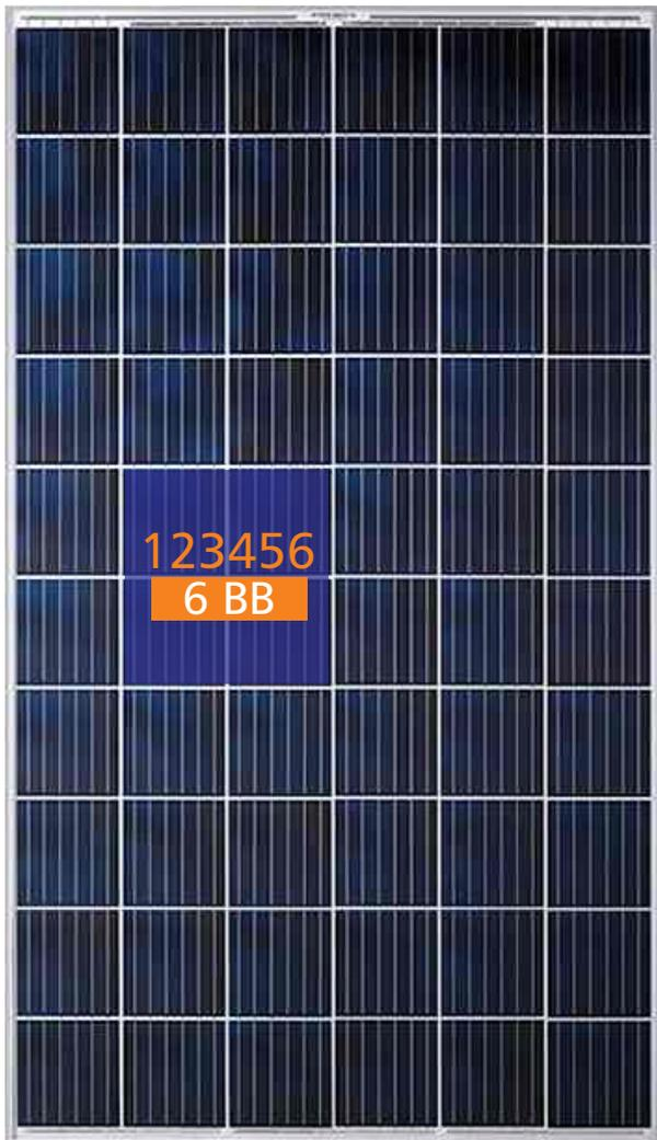
New 6 busbar cell design for more power and better reliability. The narrower distance between the busbars allows better flow of electrons and reduces power loss. Can decrease the risk of the cell Micro cracks and broken finger.
